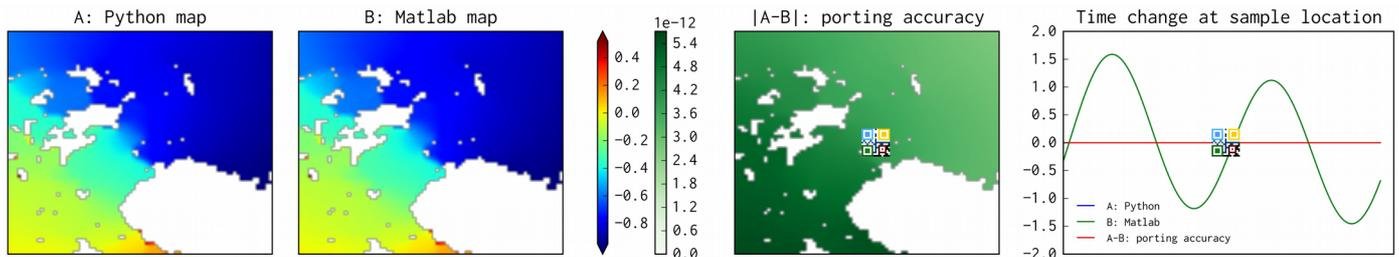
*Left* The three maps show results for the same moment in time calculated with the product Python code (A), with the given **MATLAB®** code (B) and their difference (B-A) *Right* The curves show that accuracy is also preserved over time at individual points in space. (Figures drawn with **matplotlib**, Python's own plotting library.)
